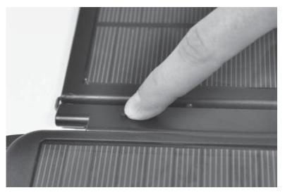
Press the connection test button on the panel link. The capacity indicator lights will stop flashing and the LED indicator on the panel link will turn off. \*You can also refer to the instruction label on the panel link.
